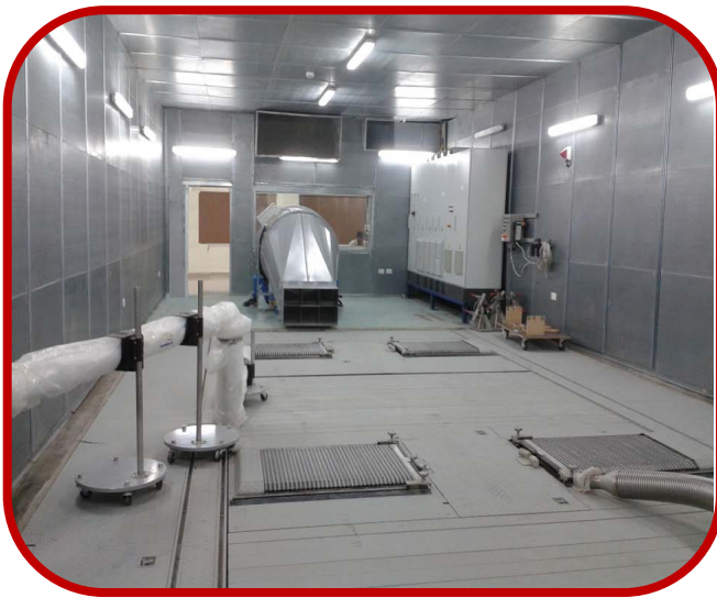
Vehicle Test Cell (Chassis Dyno.)
