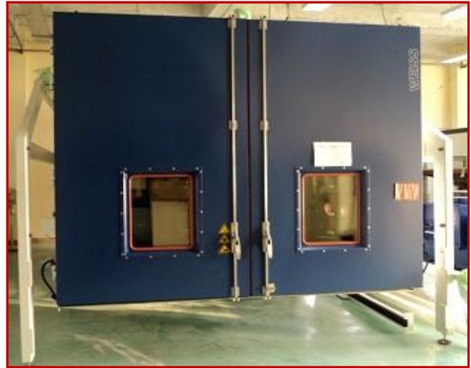
Large Climatic Chamber for Integration with Large ED Shaker
